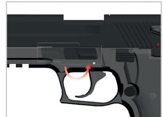
5. Rotate the takedownlever backwards. (180°). Reinstall threaded cap (only for model GSG firefly SD).
