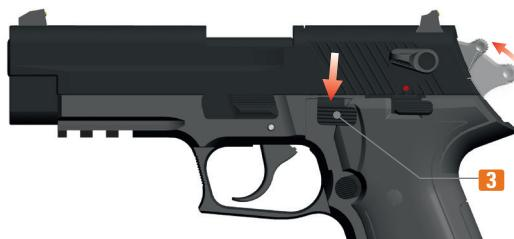
3. The pistol can now be decocked using the decocking leve **3**. It is then loaded, decocked and ready for firing in the double action (decocked) mode.
