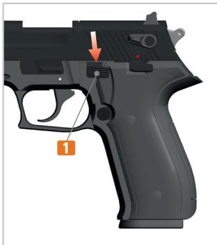
1. Engage the safety and press the decocking lever **1** to decock the hammer.
