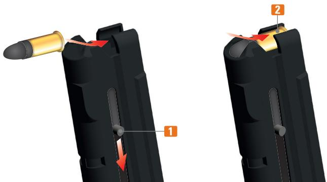
1. Pull down the feeder taps **1** of the magazine and insert the cartridge **2** into the magazine (push it to the back stop of the magazine as shown).
