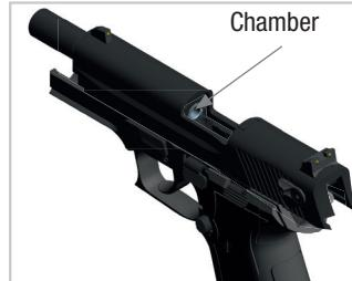
3. Pull the slide back until it stops. Hold it in this position to allow the cartridge to be ejected. Check (visually and manually with appropriate aid) to ensure that the cartridge has been ejected and the chamber is empty.
