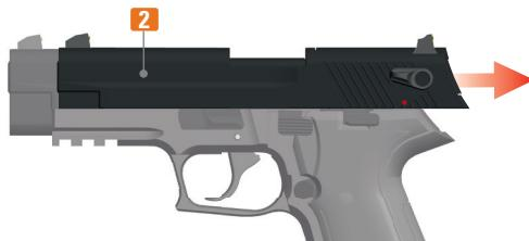
2. Pull the slide **2** back until it stops and allow it to slide forward.
