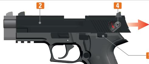
2. **Single Action Mode:** Now pull the slide **2** back until it stops and then let it slide forward again by operating the slide catch lever **5**. Secure the gun with the safety lever **4**.
