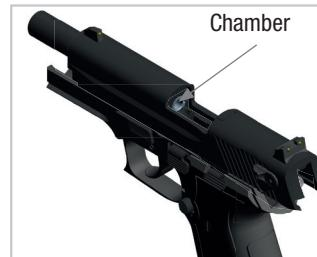
3. Verify (visually or with a tool) that there is no projectile, cartridge, case or foreign body in the barrel bore or chamber.
