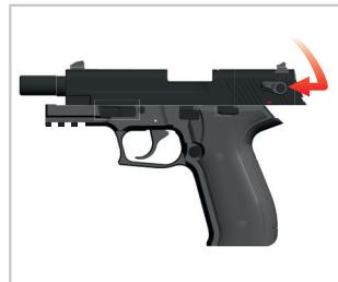
3. Bring it down until the slide guide can click into the frame guide. Slowly move the slide forward until it is closed.
